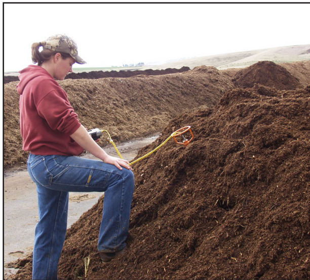
Measuring internal pile temperature on a mortality compost trial at the WSU compost yard.
